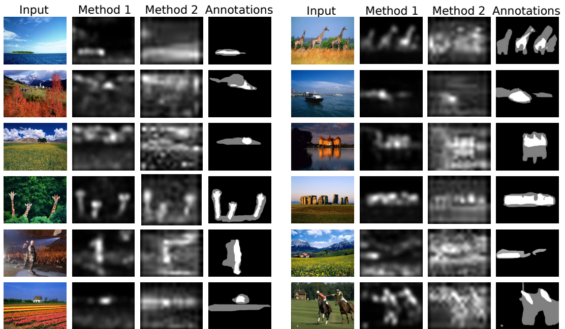
Figure 2.2: Examples of saliency detection. For input images we show the result of applying Method 1 (Hou and Zhang, 2007) and Method 2 (Itti and Koch, 2000). In order to obtain a ground truth of the saliency, all the images were labelled by four annotators. The black area of the annotations corresponds to non-salient regions, the grey area was a region identified as salient by at least one of four annotators, and the white area is the region selected by all four annotators. Figure reproduced from (Hou and Zhang, 2007).
