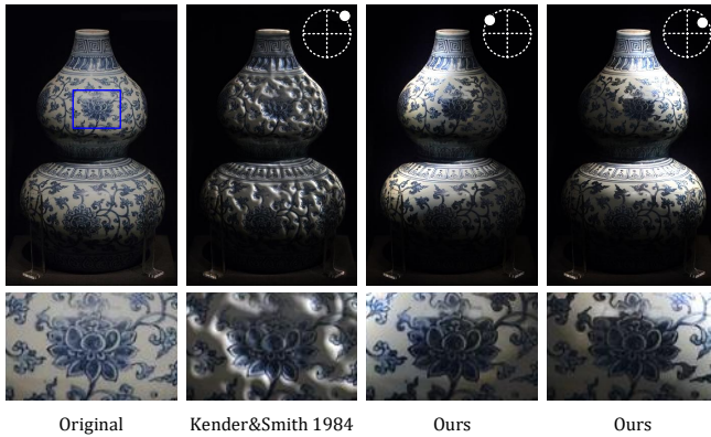
Fig. 12. Comparison with height-to-normal-based relighting. We compare our algorithm to the shape-from-shadow transform, where the per-pixel intensity is used as the height map.
