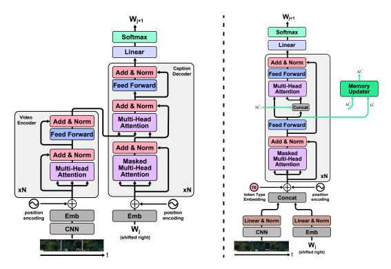
Figure 2: Overview of our captioning models. The left model is based on the vanilla transformer proposed by Zhou *et al.* [37], while the model on the right is based on the transformer with recurrent memory module [15].
