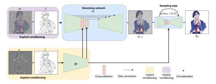
Figure 2. Overview of our proposed user-guided line art colorization. The framework is composed of two main components: a denoising model  $\epsilon_{\theta}$ , which learns to generate a denoised image, and an application-specific encoder  $g_{\theta}$  for extracting user color scribbles information.
