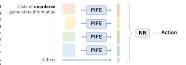
Fig. 1. Our permutation invariant deep reinforcement learning model. Unordered input data is processed by PIFE that extracts the abstract values which is passed to NN.
