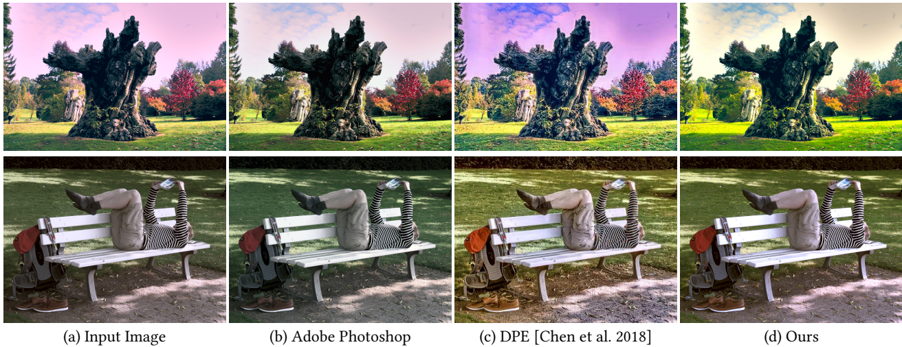
Figure 4: Comparison of automatic enhancement results with existing approaches. More results are in the supplementary materials. The top image is “Sheffield Park and Garden 22-10-2010” by Karen Roe licensed under CC BY 2.0. The bottom image is “Strasbourg” by francois schnell licensed under CC BY 2.0.
